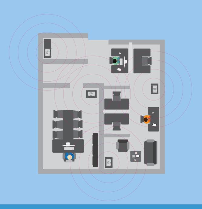
Channel utilisation and neighbouring channel interference within the coverage area needs to be assessed to determine what the optimal wireless frequencies are.
